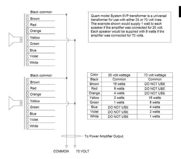
\*Note:Each unused transformer tap must be insulated from each other and from ground.
